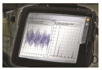
Using ExpertALERT's "User Defined Point" feature, special tests performed using RTA can be associated with machinery in your condition monitoring program and are accessible from the ExpertALERT tree. Click on the test and ALERT RTA (in viewer mode) will open up and display the appropriate data.
